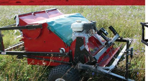
Tipping the 600 litre hopper (left) to bag off heather seed from 3 chutes ready for further cleaning and drying.
