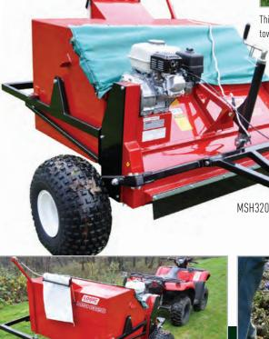
This model features a 600 litre capacity hopper with tipping rope and single pivot point. The contents would typically be tipped onto a tarpaulin or sheet for further processing before drying and cleaning (as shown right).
